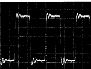
25 IC307 58pin (F128) 5.8Vp-p, 0.17μs
